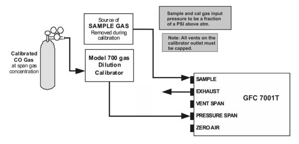
Figure 9-5: Pneumatic Connections – Option 50H: Zero/Span Calibration Valves
